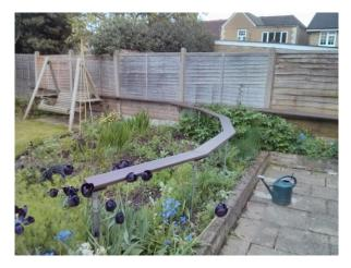
The idea is to use small diameter stainless steel tube rather than the more conventional timber fence posts and good quality decking timber. There is a single track 3m radius oval with a reverse curve on the free standing side, and a fence-mounted 6m long run of sidings for stock and steaming up.
